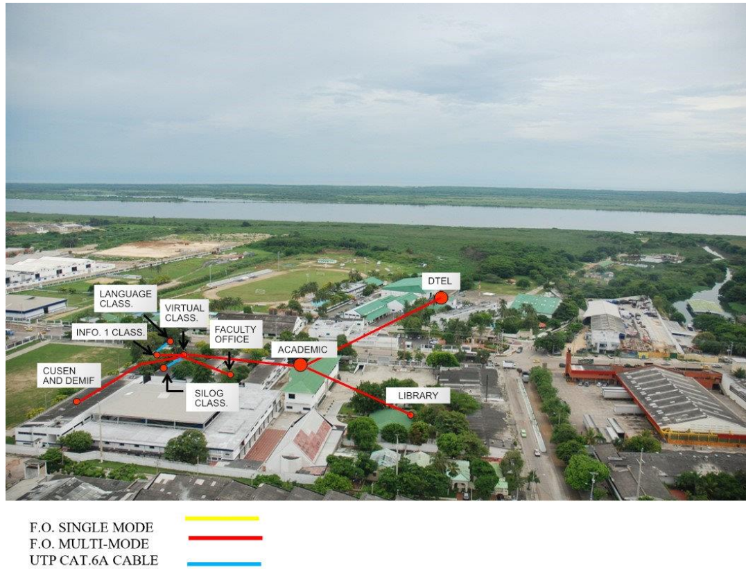
Figure 1. Wiring in the Academic Department.
