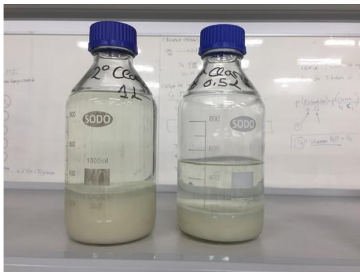
Figure 4. Detail of phase separation before clarification (upper image) and after clarification (lower image).
