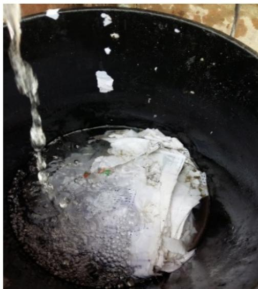
Using a Hobart mixer, the 75 g bond paper was homogenized by shredding it and adding water until a uniform consistency was achieved, as shown in Figure 3.
