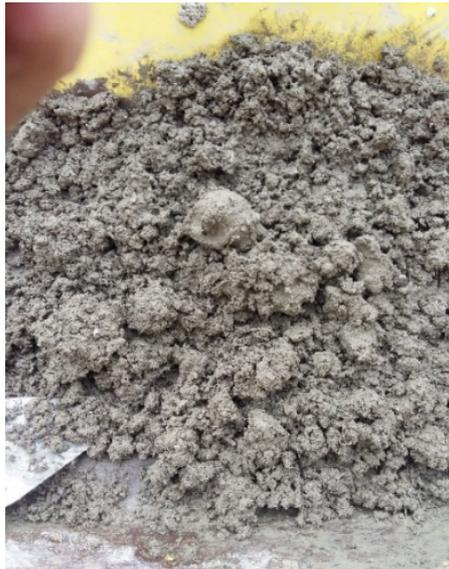
Consequently, the mixture is placed in wooden molds and then beaten with a rubber hammer to get the material to settle properly and eliminate excess air. After ensuring the correct distribution of the material and covering empty spaces, the mold is removed, leaving the ecological bricks as shown in Figure 6, which also shows the presence of a metal plate used to level the upper face that will receive the load in the compression tests.
