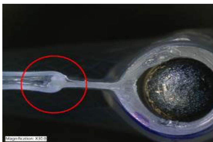
Figure 16. Welding rejected by visual inspection
