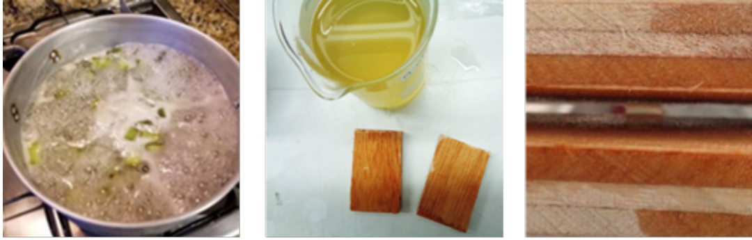
Figure 7. Mucilage cooked at 80 ° C, and its effectiveness as an adhesive.
