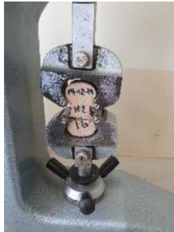
Figure 19. Tensile stress rupture test scheme.
