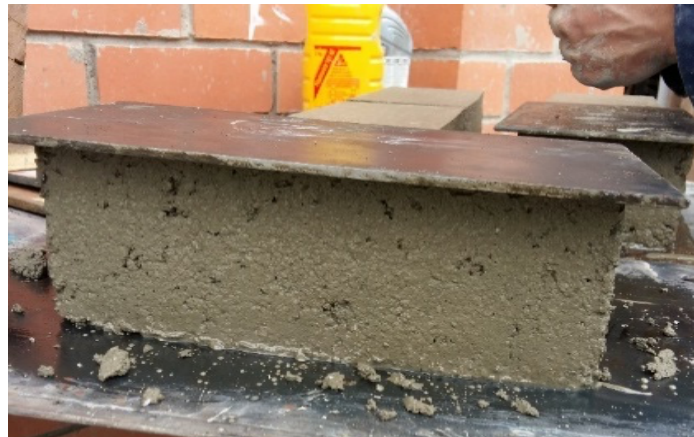
Figure 6 Demolded bricks with presence of leveling plate
